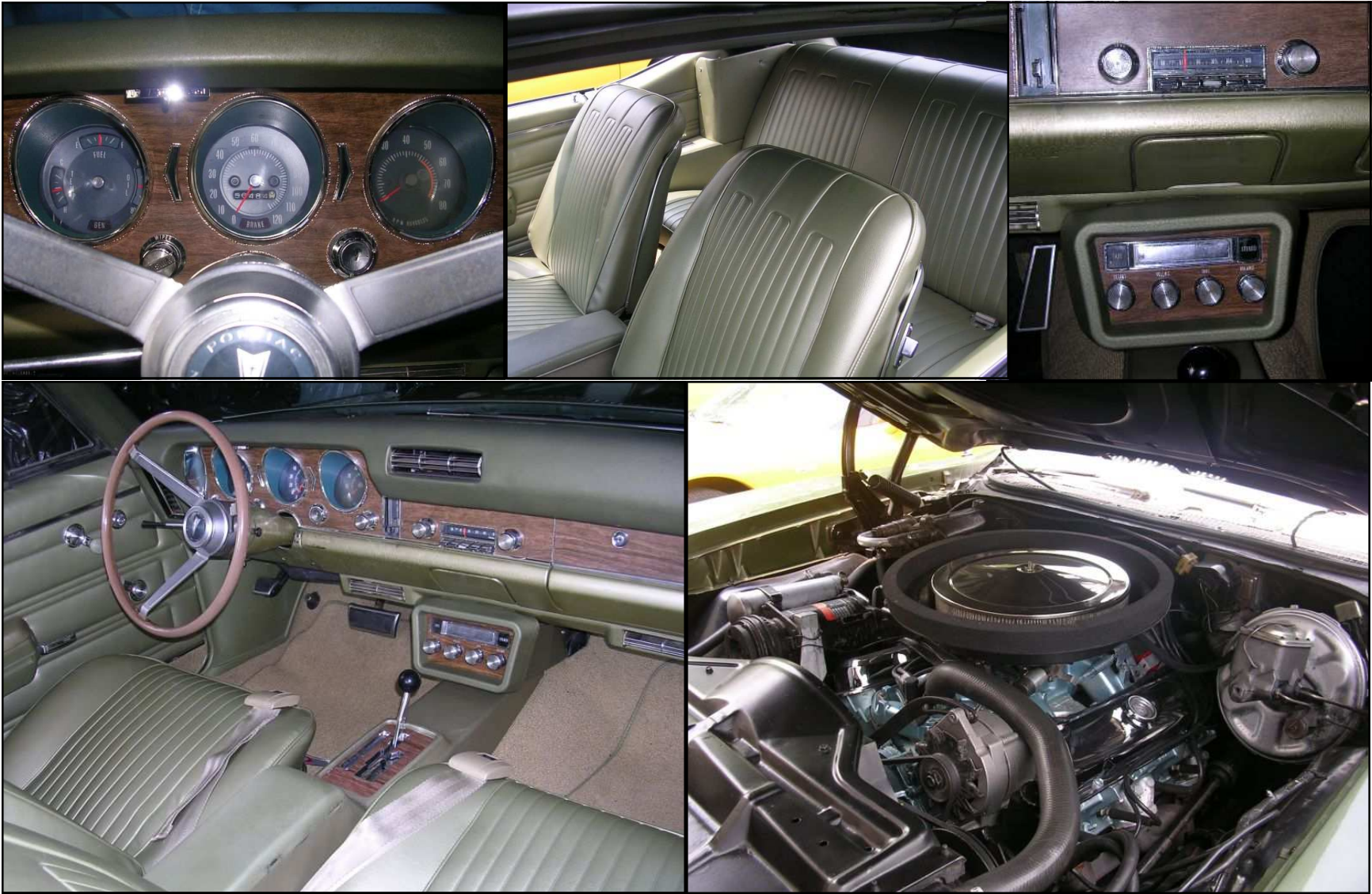
Here are spot shots of my GTO convertible and all of it's options. Its a Royal Bobcat 428 HO Ram Air, console, turbo hydramatic with Hurst Dual Gate, 3.55 positraction, tac and gauges, air conditioning, 8 track, am/fm, hid-a-way head lights, front power disc brakes, power steering, Rally II wheels, wood sport steering wheel, remote side view mirror and tinted windows.
